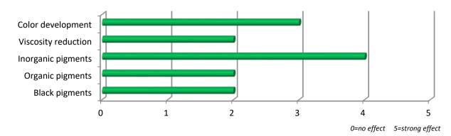
LINIQ®SPERSE P-904 is a wetting and dispersing additive in unsaturated resin systems and adhesives. It's no silicone dispersant. The additive prevents the flooding/floating and settling of pigments and fillers in epoxy and VE/UP-based laminates. Reduction in the flooding/floating of colored pigments in gel coats. And it can reinforce the rheological effectiveness of pyrogenic silica to increase and stabilize the thixotropic behavior.
